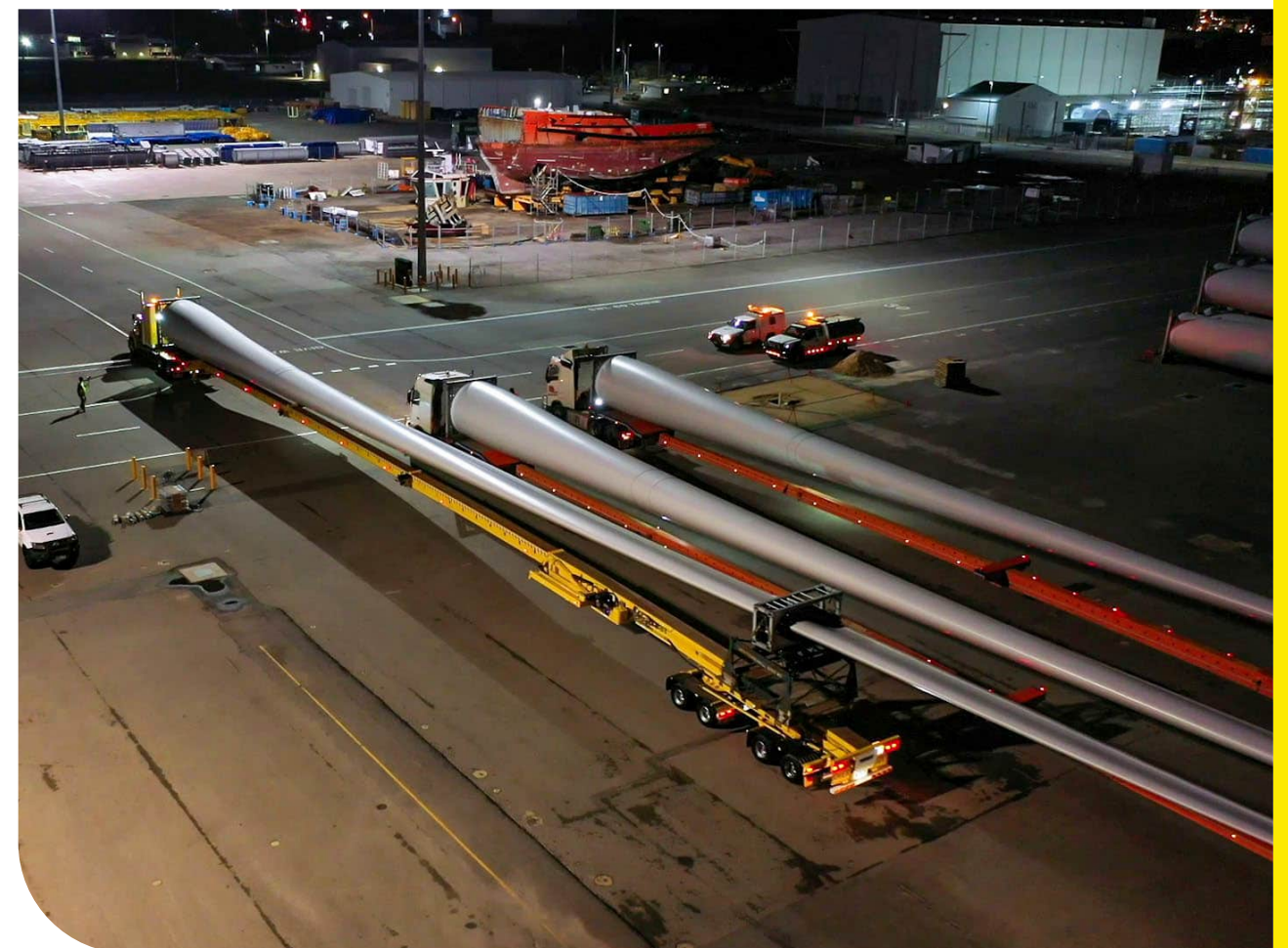
Above: Extendable blade trailers loaded with 75m blades for the Yandin project in Western Australia.
