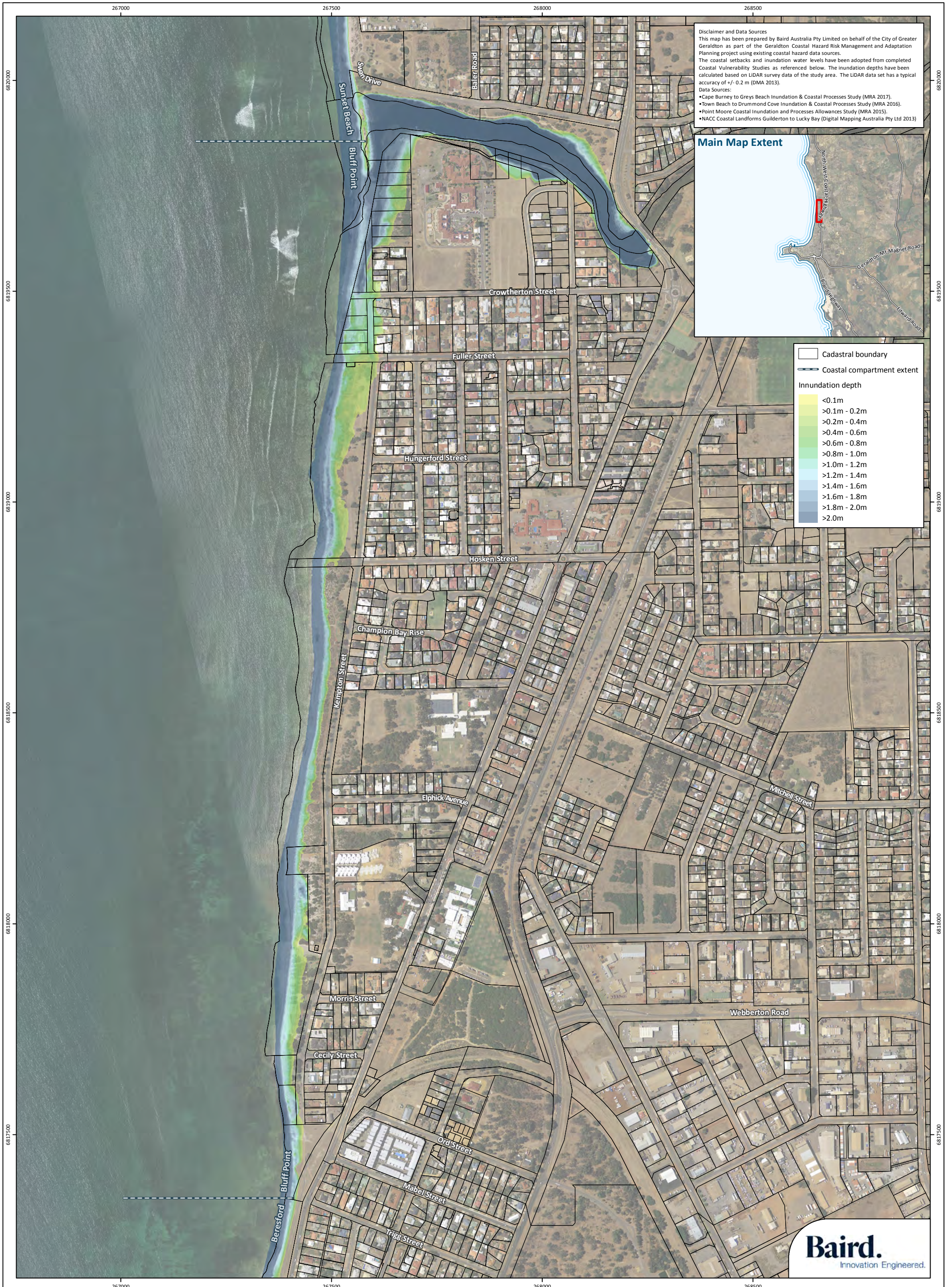
Figure 4 of 12 Coastal Hazard Mapping : 2110 Coastal Inundation Depth 100yr ARI Event, Bluff Point Project: Geraldton CHRMAP Project Client: The City of Greater Geraldton
