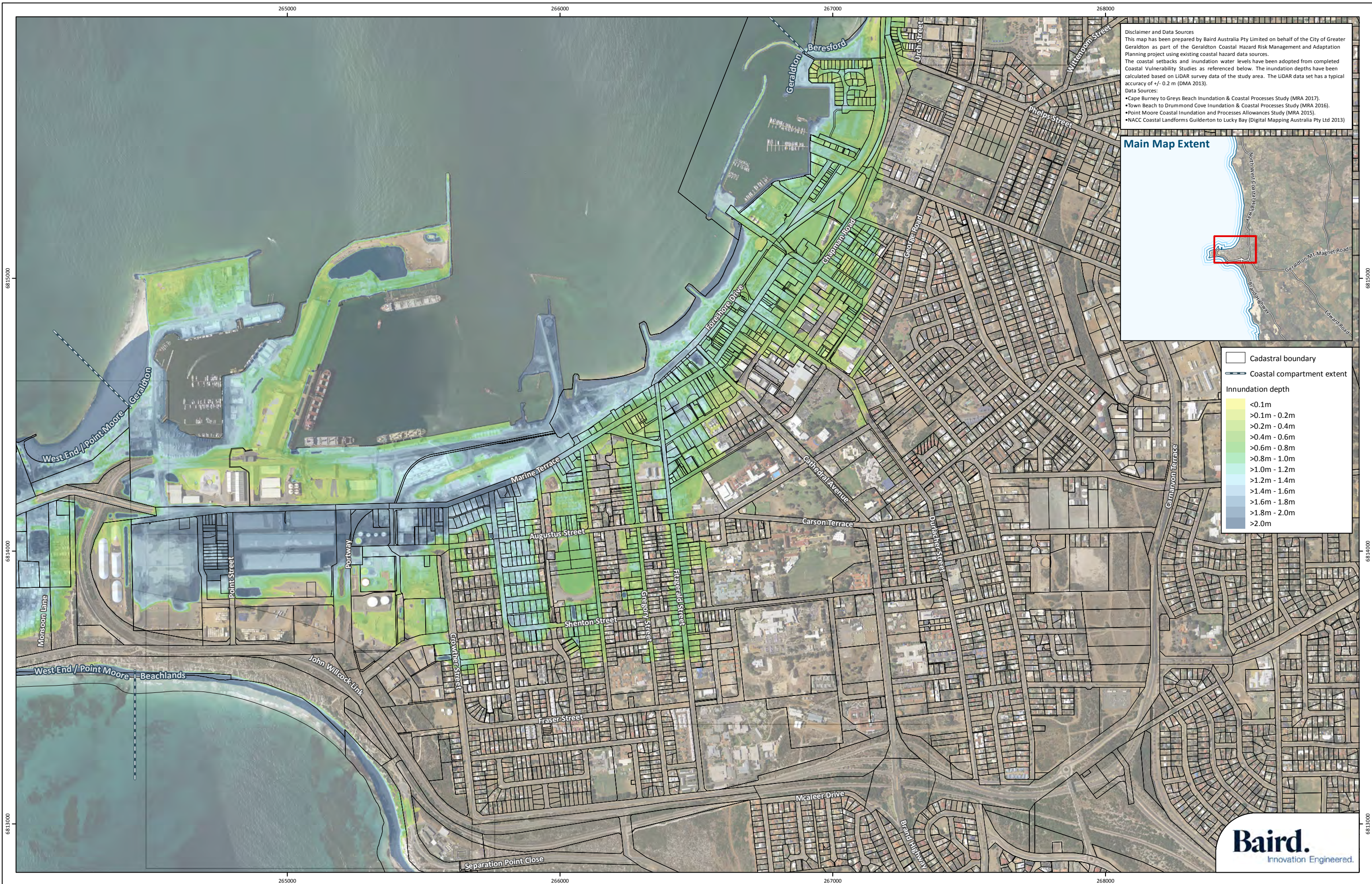
Figure 6 of 12 Coastal Hazard Mapping : 2110 Coastal Inundation Depth 100yr ARI Event, Geraldton Project: Geraldton CHRMAP Project Client: The City of Greater Geraldton
