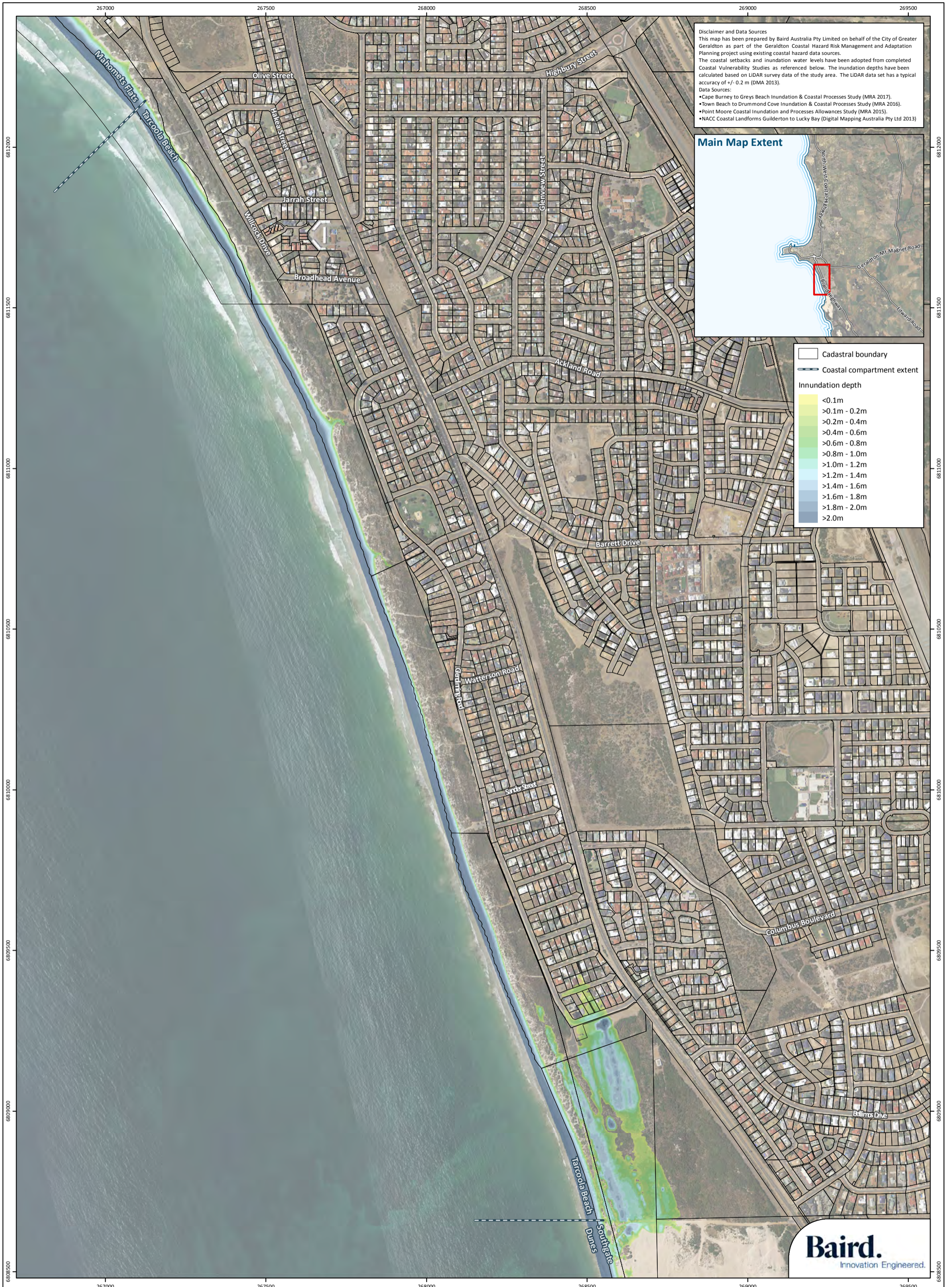
Figure 10 of 12 Coastal Hazard Mapping : 2110 Coastal Inundation Depth 100yr ARI Event, Tarcoola Beach Project: Geraldton CHRMAP Project Client: The City of Greater Geraldton
